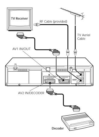
The AV2 IN/DECODER connector can be used as an input terminal for an external decoder (descrambler). Simply connect a decoder and you can enjoy the variety of programming that is available through scrambled channels.
